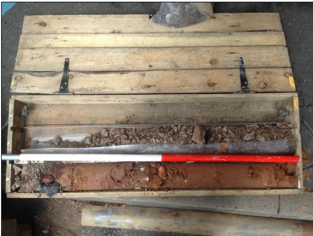
Plate 10: BH 1302, from ground level to 1.5m BGL
